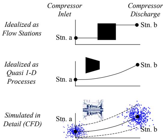
**Fig. 1: Application of work potential methods at various levels of analysis fidelity.**
