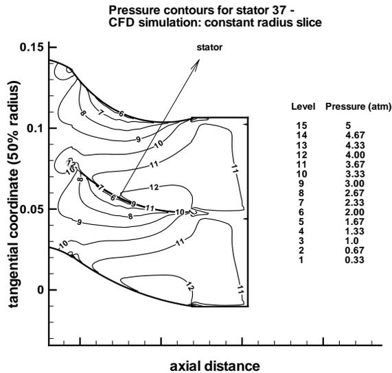
**Fig. 12 Pressure contours from stator row 37 (constant radius view).**
