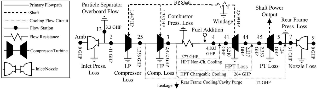
**Fig. 4: Cycle model schematic with annotation of major loss mechanisms and estimates on GHP at each flow station for SLS full power operating conditions.**
