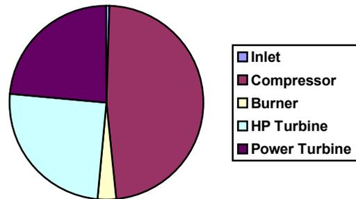
**Fig. 11 Percent of lost shaft work in power turbine (sorted by component).**
