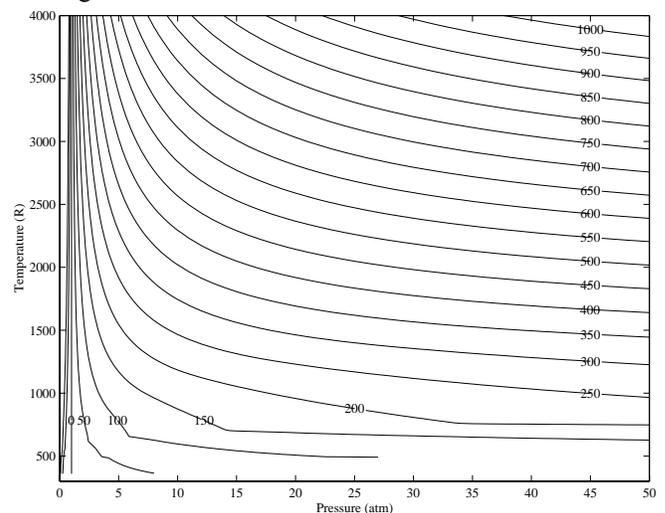
Fig. 3: Contours of mass-specific gas horsepower (HP/pps) for stoichiometric mixtures of Jet-A and air.
