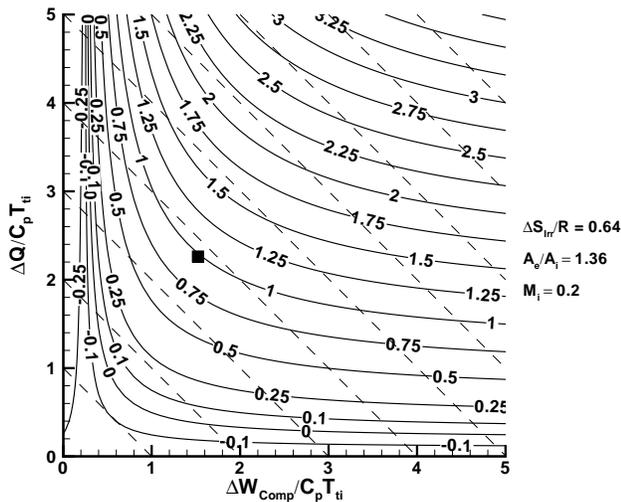
Fig. 7 Burner heat addition and compressor work addition shaft work contours ( $\Delta W_{shaft}/C_p T_{ti}$ ).
