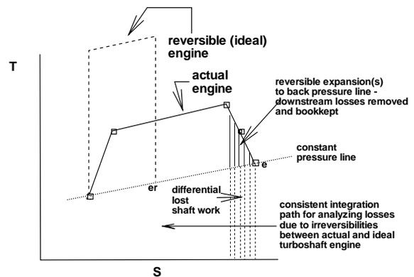
Fig. 5 T-S diagram showing actual and ideal engine cycles with intermediate loss cycles.
