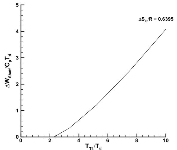
Fig. 8 Maximum shaft work versus burner exit total temperature ratio for a constant irreversibility.
