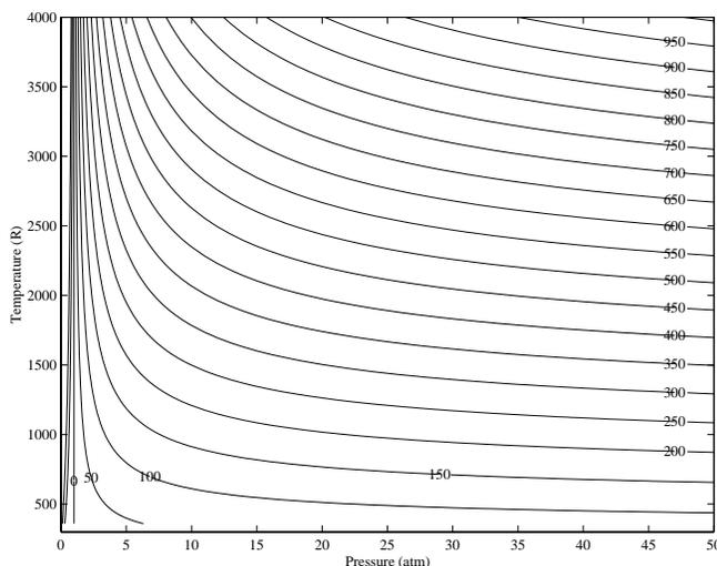
Fig. 2: Contours of mass-specific gas horsepower (HP/pps) for air.
