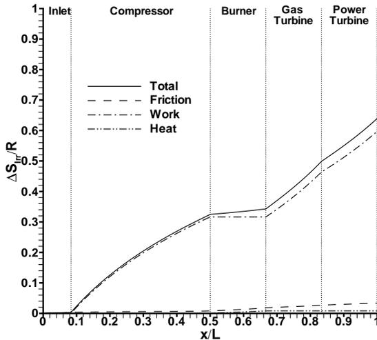
**Fig. 10 Mechanism and component irreversible entropy increases.**
