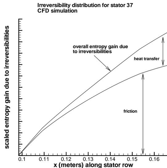
**Fig. 13 Entropy distribution due to irreversibilities along stator row 37.**
