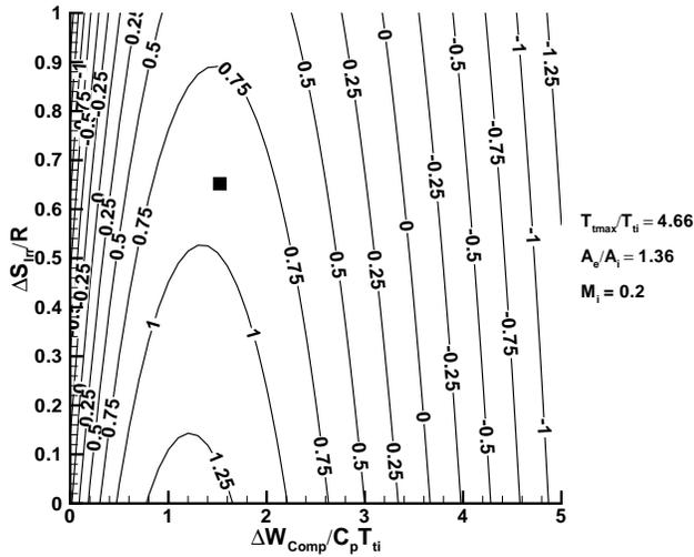
**Fig. 9 Irreversible entropy increase and compressor work addition shaft work contours.**
