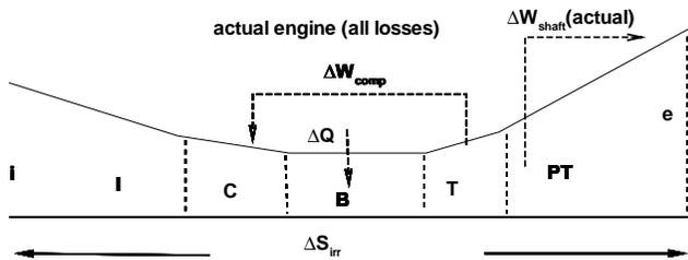
Fig. 6 Turboshaft engine schematic and energy interactions.
