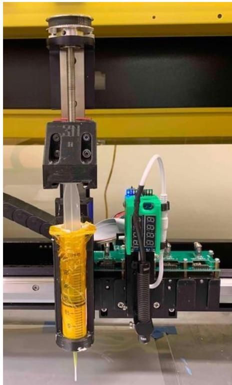
Fig. 4. The 3D printer fully set up for the experiment. The print head with syringe loaded is on the left and the UV light is to the right.
