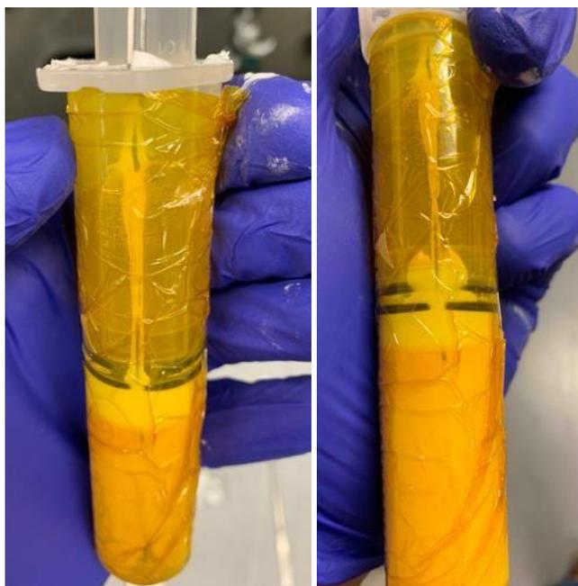
Fig. 2. (left) loaded syringe with paperclip pre-mixing. (right) loaded syringe with paperclip post mixing.
