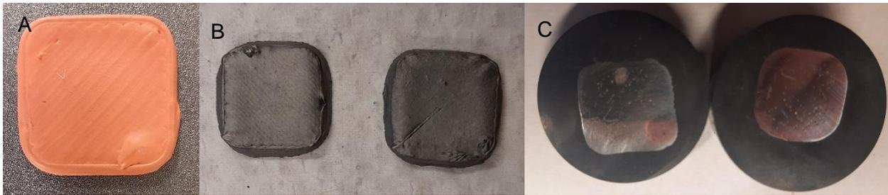
**Figure 1:** **A:** Sample after printing. **B:** Samples after furnace processing. **C:** Samples mounted and ground for hardness testing
