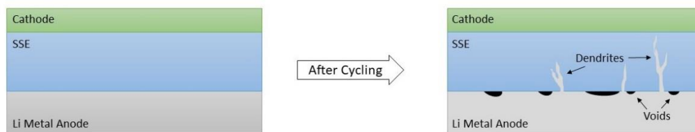
Figure 2: On the left is a simple schematic of a cross-section of a solid-state battery (SSB). As illustrated on the right, charging and discharging the SSB can cause voids and dendrite growth at the interface between the lithium anode and the solid-state electrolyte (SSE).
