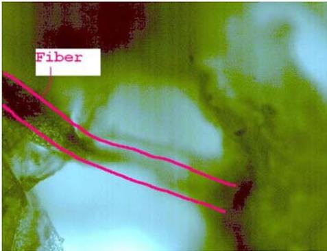
**Figure 23: Hardwood fiber across pore. Fiber content = 20% HW.**
