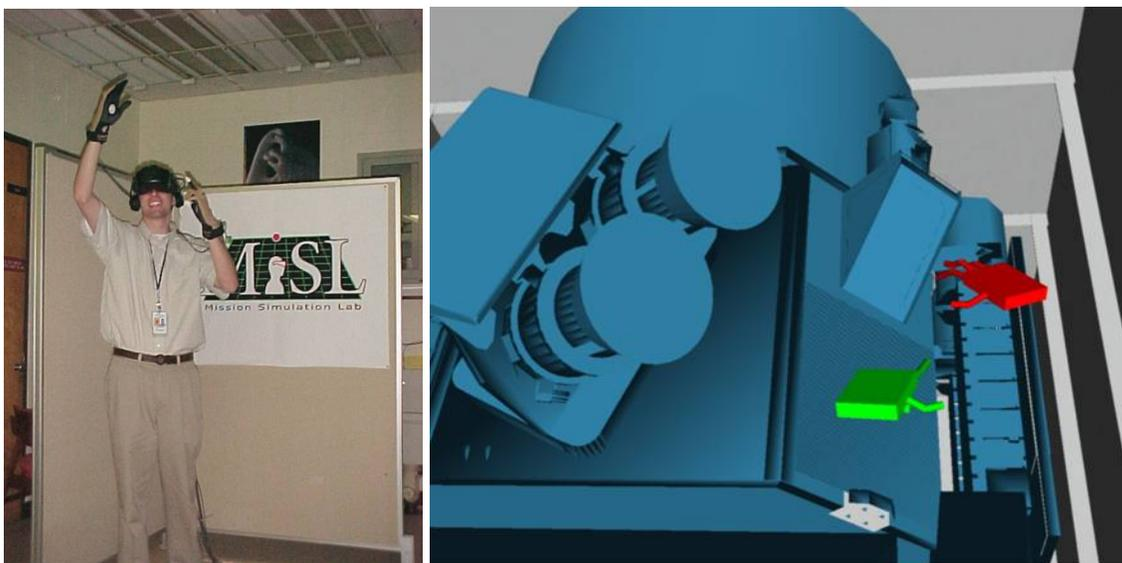
**Figure 5: (a) A MiSL engineer attempts to reach the CALIPSO launch locks, and (b) the user's view.**
