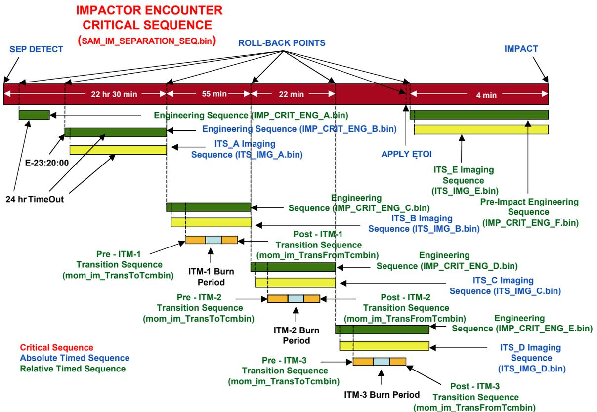
Figure 3. Impactor encounter sequence design schematic
