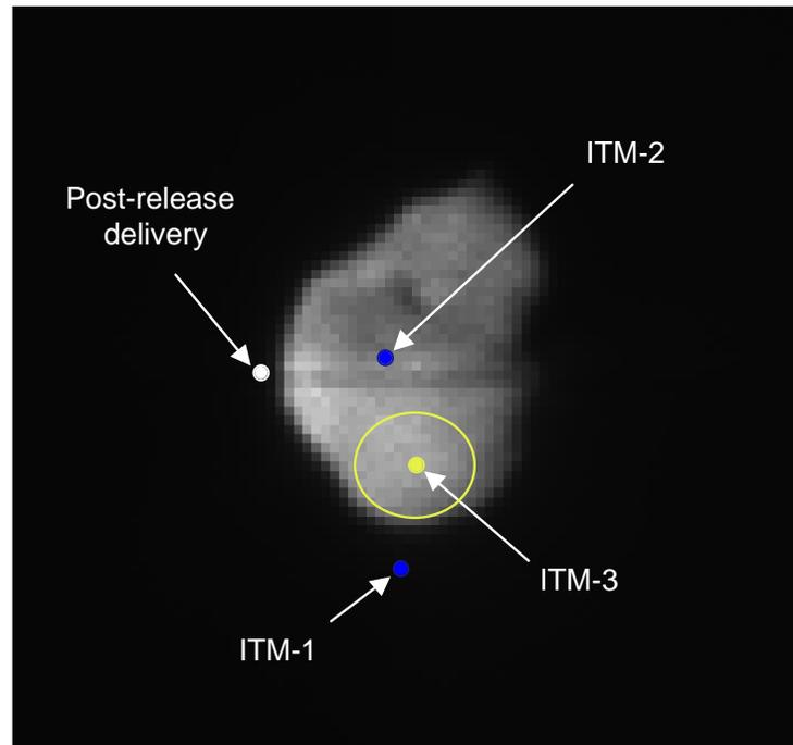
**Figure 6.** Performance of ITMs shown with respect to an AutoNav image taken just prior to ITM-2. Range is approximate 21,000 km. The CB of this image was located within a few pixels of the ITM-2 predicted intercept location
