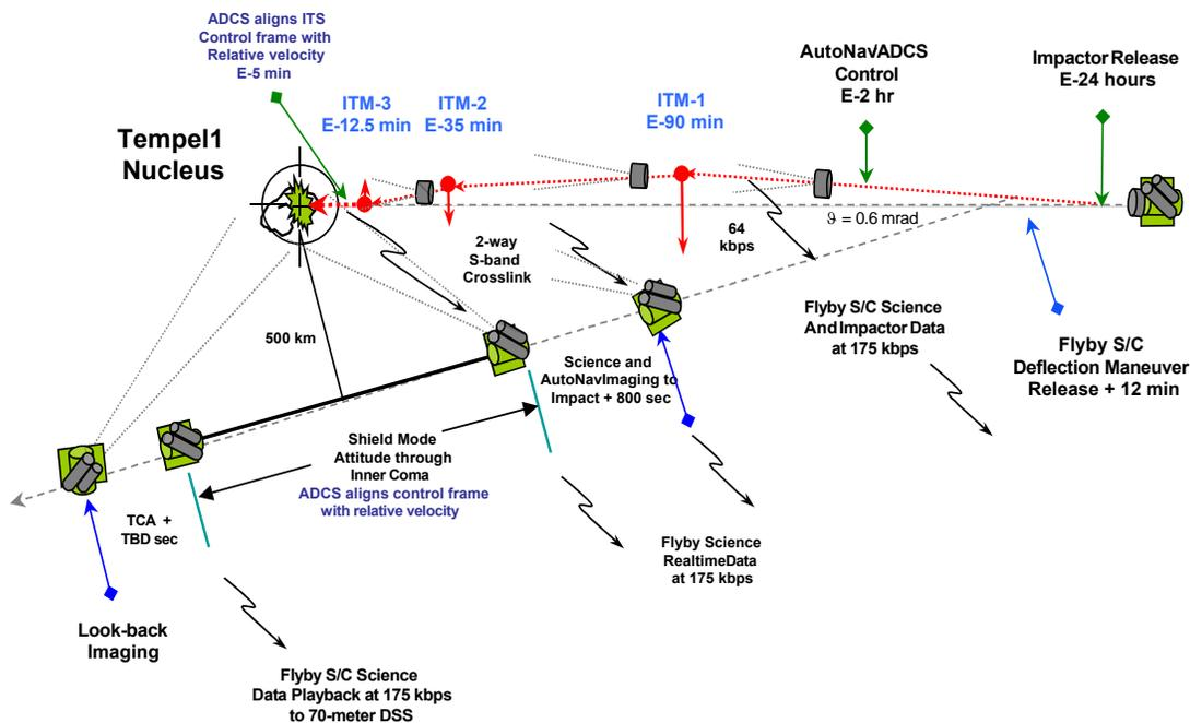
**Figure 1.** Schematic of Deep Impact Encounter with comet Tempel 1**1.2.Impactor Spacecraft Flight System**
