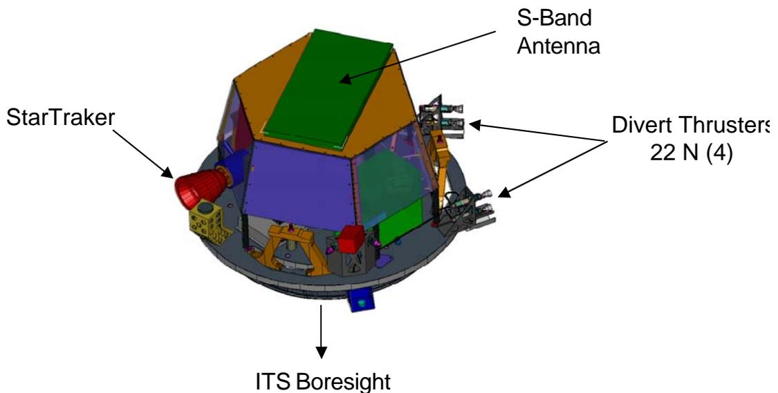
**Figure 2.** Impactor s/c flight system configuration<sup>1</sup>
