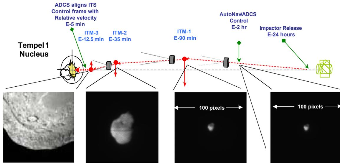
**Figure 5.** Sequence of images taking during the AutoNav/ADCS closed-loop operations
