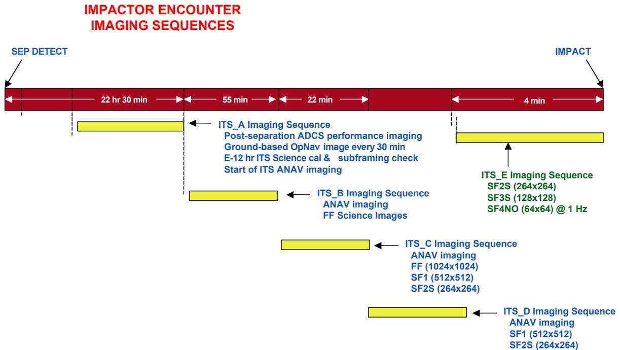
**Figure 4.** ITS imaging subsequence layout
