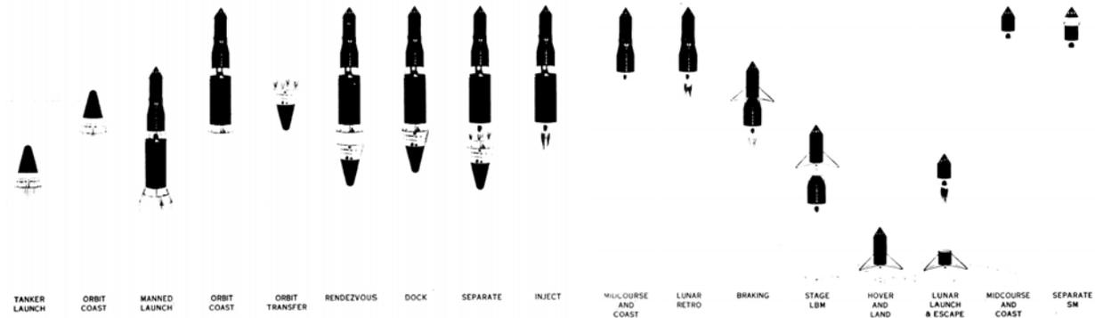
**Figure 2. Earth orbit rendezvous concept of operations.**<sup>3</sup>
