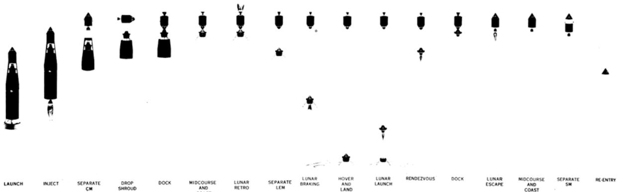
Figure 1. Lunar orbit rendezvous concept of operations.<sup>3</sup>
