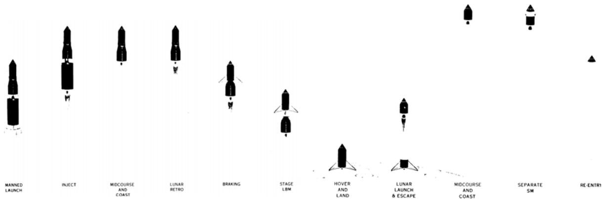
**Figure 3. Direct flight concept of operations.**<sup>3</sup>
