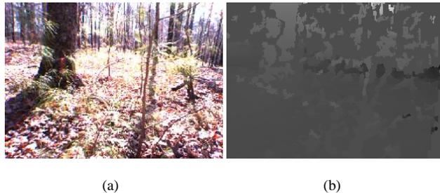
Figure 1: Input from one stereo pair. (a)RGB image from one camera; (b)Height map from stereo.
