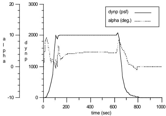
Figure 8a - Dynamic Pressure and alpha vs. Time for Final Design
