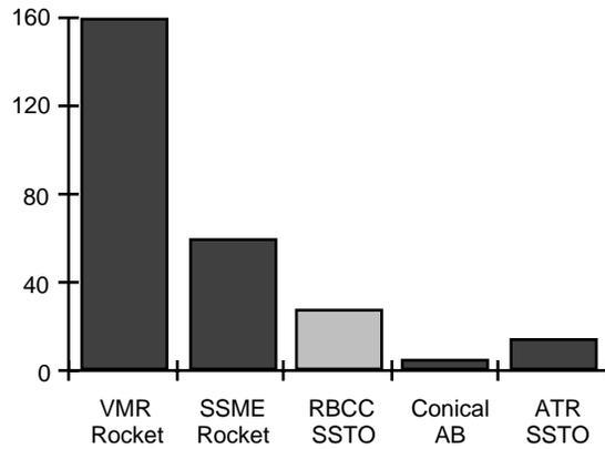
Figure 14 - Engine Installed T/W<sub>0</sub> Comparison
