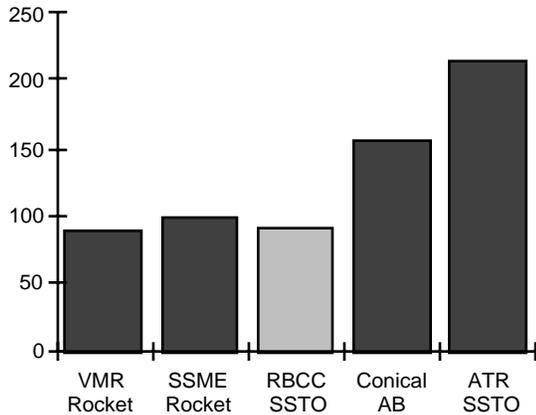
Figure 12 - Dry Weight (klbs) Comparison
