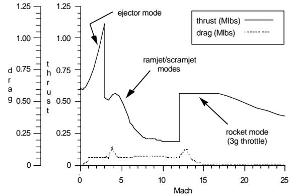
Figure 10 - Thrust and Drag vs. Mach for Final Design
