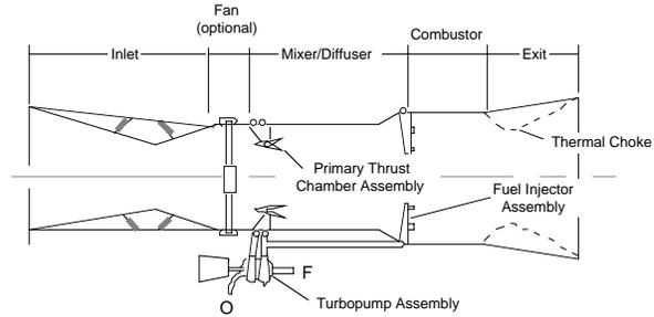
Figure 4 - RBCC Engine Layout
