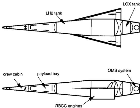
Figure 2 - RBCC SSTO Configuration
