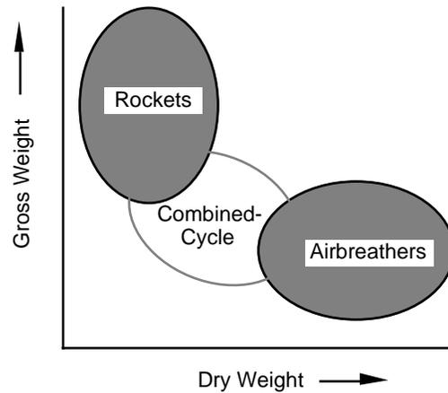
Figure 1 - Potential for Combined-Cycle Propulsion
