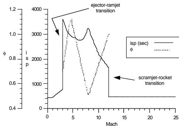
Figure 9 - Isp and  $\phi$  vs. Mach for Final Design
