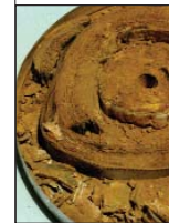
All motion pictures made before 1950 were printed on a cellulose nitrate base that deteriorates after exposure to air.
