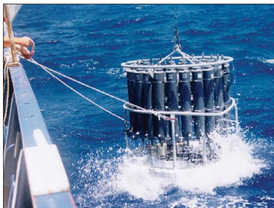
Researchers sample ocean water with a CTD-rosette, which consists of an aluminum frame, a sensor system and 24, 10-liter PVC sampling bottles. The equipment’s sensors transmit real-time information on the physical and chemical structure of the water via a conducting cable.
