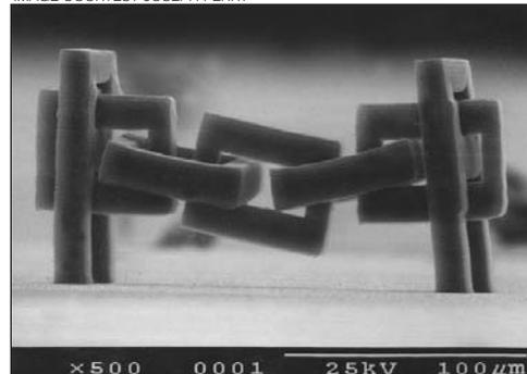
**This microchain structure fabricated with the "two-photon 3-D lithography" process is an example of a structure that would be difficult to produce layer-by-layer with 2-D lithographic processes. The links are topologically connected, but not directly anchored to the surface.**
