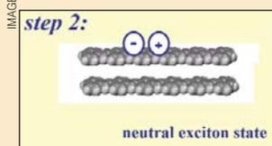
**A two-step charge recombination process begins when two initially separated charges combine to form a loosely bound, charge-transfer (CT) state. That then decays down to a lower singlet or triplet neutral exciton state.**
