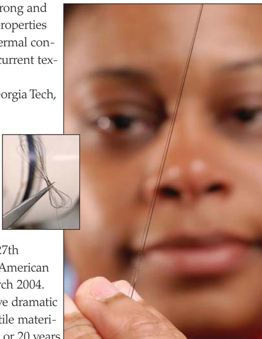
**Lab coordinator Marilyn Minus examines a composite fiber made of single-walled carbon nanotubes and polyacrylonitrile – a carbon fiber precursor. The composite fibers (inset) are stronger, stiffer and shrink less than standard fibers.**
