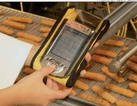
**A wireless handheld computer system under development at GTRI allows personnel to collect, retrieve and analyze a range of information from any location in a food processing plant, enabling closer control of production processes.**
