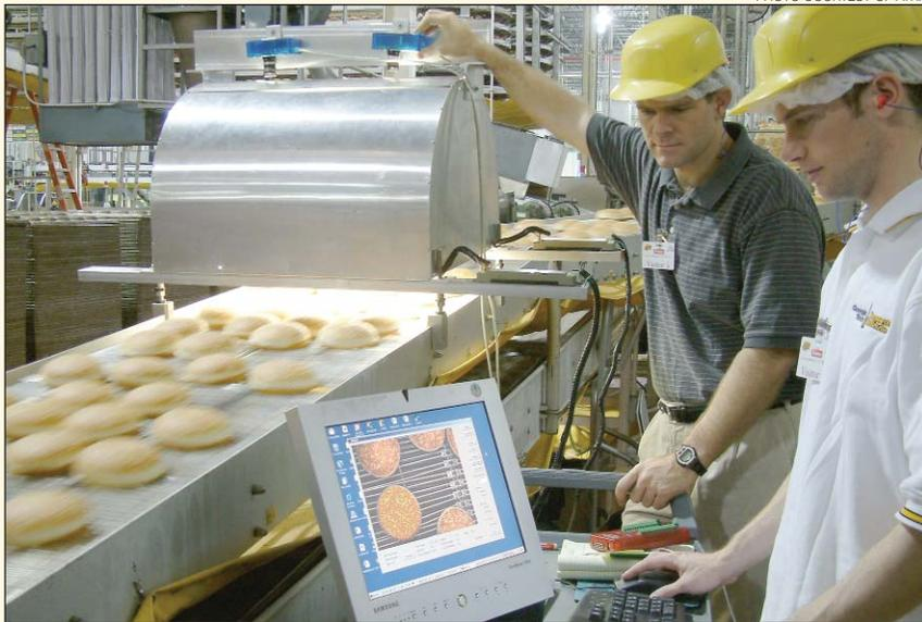
**An automated product-inspection prototype is under development by GTRI researchers working with Flowers Bakery in Villa Rica, Ga. Researchers are introducing continuous imaging technology to the large-scale production of sandwich buns for fast-food restaurants, which hold to exacting product specifications.**
