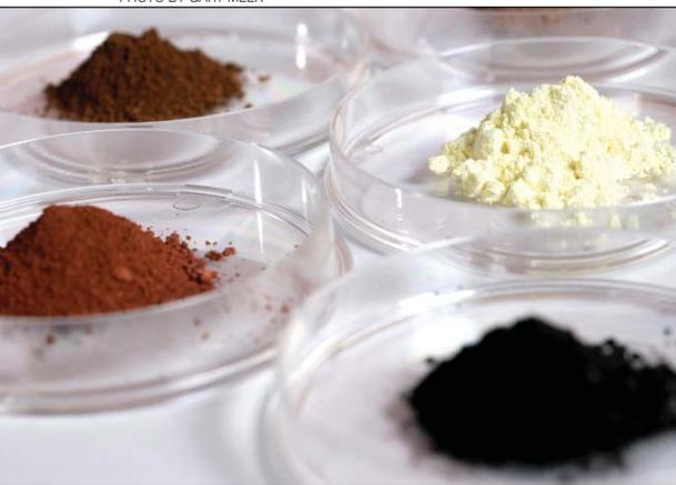
**Oxides of the rare-earth elements cerium (Ce), terbium (Tb), and praseodymium (Pr) can produce hydrogen from water vapor and methane in continuous “inhale and exhale” cycles.**
