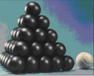
**In pebble-bed modular reactors, a cylindrical vat is filled with billion-ball-sized “pebbles” packed with graphite that contains thousands of uranium specks called “microspheres.”**
