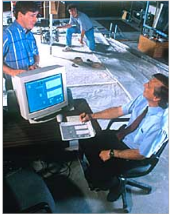
Using a pit containing 50 tons of damp sand, Georgia Tech researchers have demonstrated they can detect seven different types of buried land mines. Dr. Gregg Larson, left, Dr. Waymond Scott, right, and graduate student Christoph Schroeder, background, are detecting the deactivated weapons by simultaneously using sound waves to create tiny soil disturbances and precision radar to measure the resulting movement.
