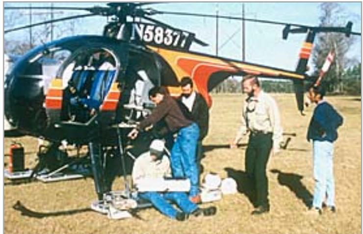
Researchers recently conducted a field test of their new power line crossarm inspection system that combines laser vibrometry and neural networks and allows workers to analyze crossarm structural integrity from the air. The process drastically reduces costs, while also boosting accuracy. ([300-dpi JPEG version - 489k](#))
