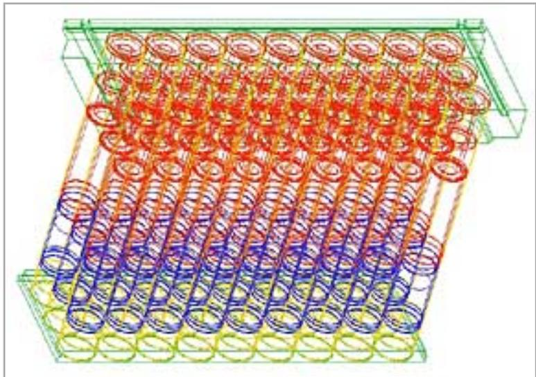
A new technology is strengthening paper fiber, while lowering the energy costs of manufacturing it. A device that is retrofitted into an existing paper machine's headbox (shown here) disperses wood fibers uniformly in all directions, strengthening the paper. ([300-dpi JPEG version - 546k](#))
