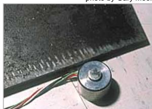
Ten strategically sized and located, force-sensitive load tiles (shown here) will be installed in the Residential Laboratory to gather footstep data from occupants. Called the "Smart Floor," the system is a natural input device that can identify and locate a person based solely on his or her footsteps. ([300-dpi JPEG version - 619k](#))
