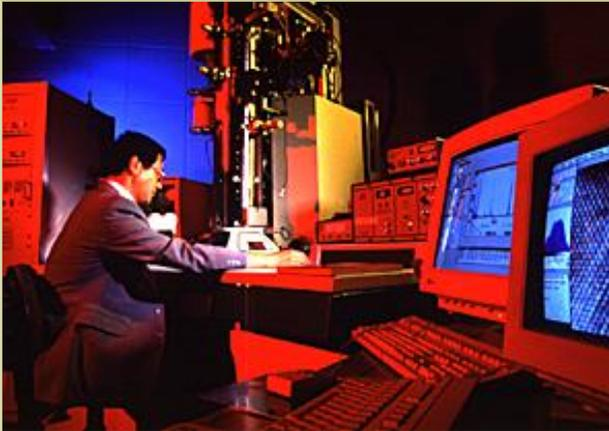
Equipment in the Electron Microscope Facility, used here by Dr. Z.L. Wang, will benefit research in nanotechnology, novel materials and structures, micro-electronics, new crystals, improved lubricants and living tissues. ([200-dpi JPEG version - 355k](#))
