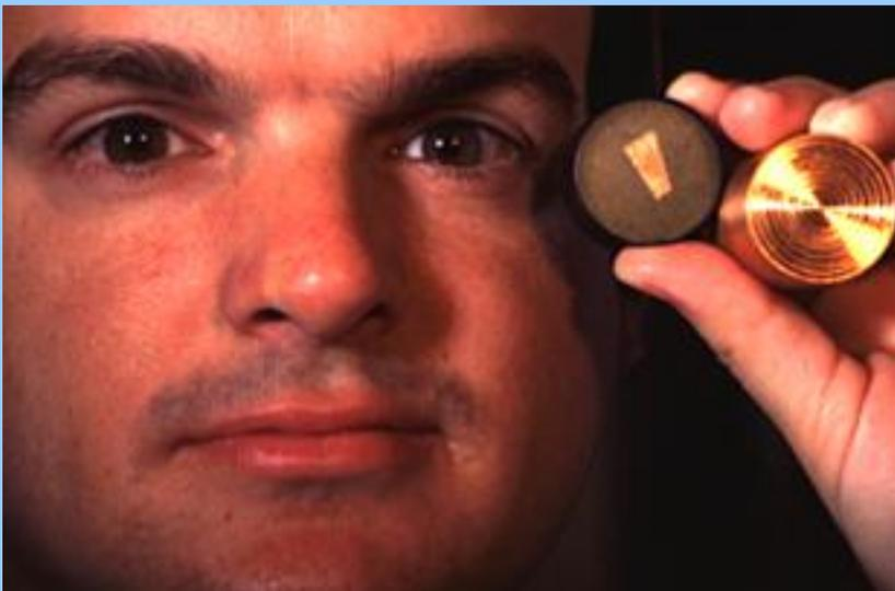
**Ph.D. student [Bob McGinty](#) displays a speck of copper, prepared for microscopic analysis of its structure, as well as a large copper piece, used for compression tests.**
