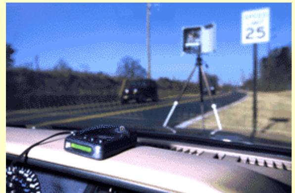
**GTRI researchers developed a transmitter and messaging system that can send a wide range of emergency warnings to motorists using advanced radar detectors, as well as a general warning to older detectors don't offer text messages.**
