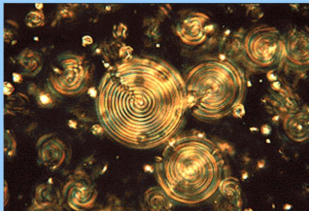
**A photomicrograph of liquid crystals suspended in glycerol helps provide information about the properties of the crystals.**
