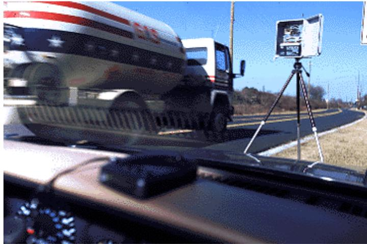
A [Georgia Tech-designed intelligent traffic system](#) uses radar detectors to alert drivers to hazards on the highway.
