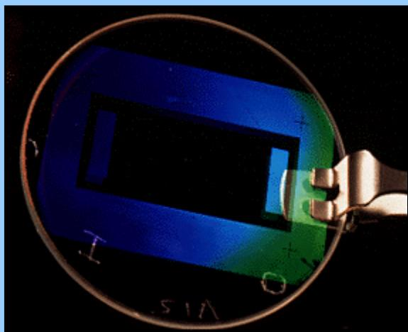
**This sensor uses laser-based technology to detect salmonella bacteria in a fraction of the time that other methods require.**
