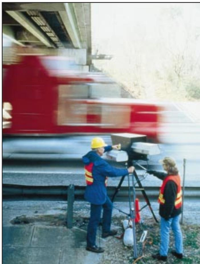
*Determining whether vehicle occupancy is increasing -- and whether that is related to changes in air pollution -- will be easier using data collected by an infrared roadside camera GTRI researchers are developing.*
