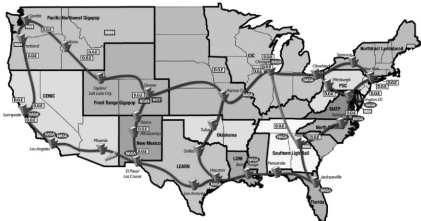
The map shows the distribution of fiber optic cable and the locations of the network's nodes. Data transmission along the network is 10 gigabits per second.
