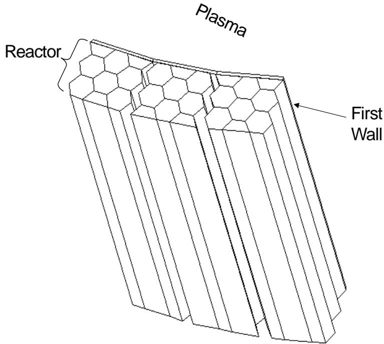
Fig. 7 Transmutation Reactor Configuration Outboard of Plasma Chamber
