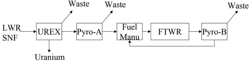
Fig. 8 Waste Processing Flow Diagram
