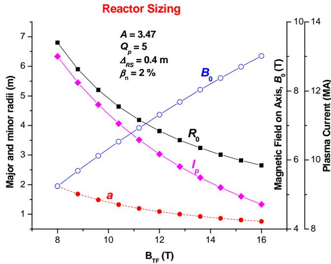
Fig. 4 Various reactor parameters ( $R_0$ ,  $a$ ,  $B_0$ ,  $I_p$ ) vs. the maximum toroidal field at the coil,  $B_{TF}$ , for a set of fixed shape and performance parameters.
