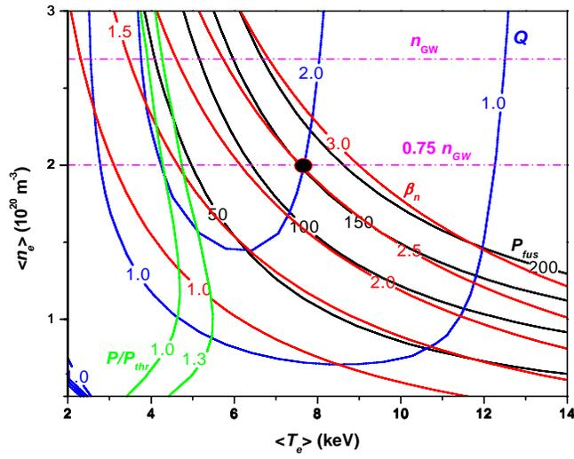
Fig. 5 POPCON Plot for the reference design of the fusion neutron source. Contours of constant fusion power,  $Q_p$ , normalized beta and  $P_{sep} / P_{LH}^{thr}$  ratio are shown. In addition, lines of constant  $\langle n_e \rangle / n_{GW}$  ratio are also shown. The reference operating point is marked by a solid circle.
