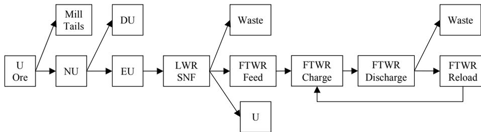
Fig. 9 FTWR Toxicity Flow Diagram
