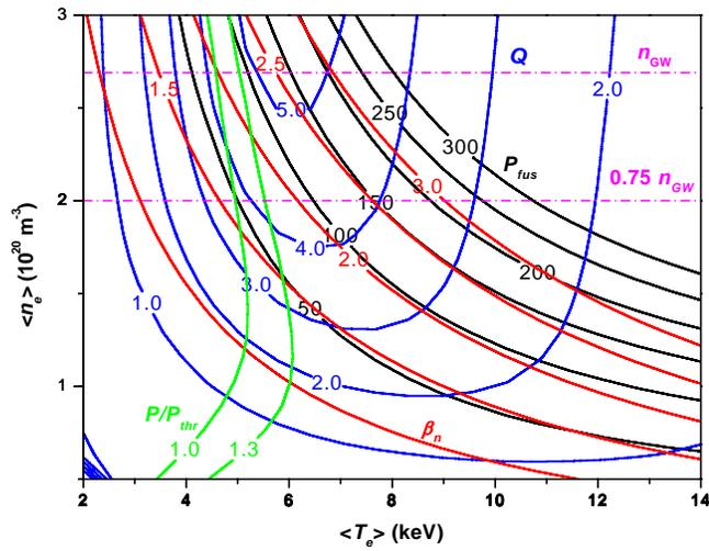
Fig. 6 POPCON plot assuming a confinement enhancement factor  $H = 1.3$
