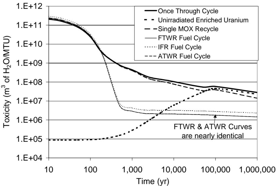
Figure 3 - Toxicity of Waste Sent to Repository per Unit Mass of LWR SNF
