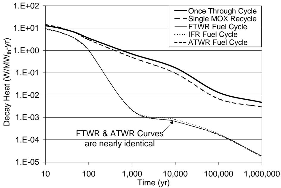
Figure 8 - Rate of Production of Decay Heat
