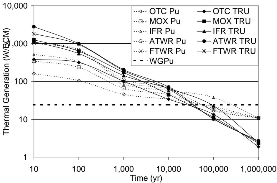
Figure 11 - Decay Heat From One Bare Critical Mass
