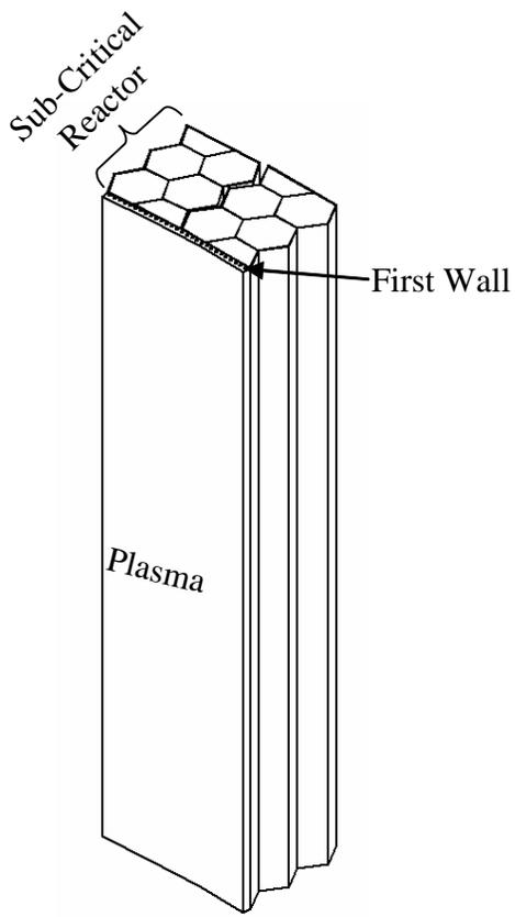
Figure 16 - Transmutation Reactor Configuration Outboard of Plasma Chamber
